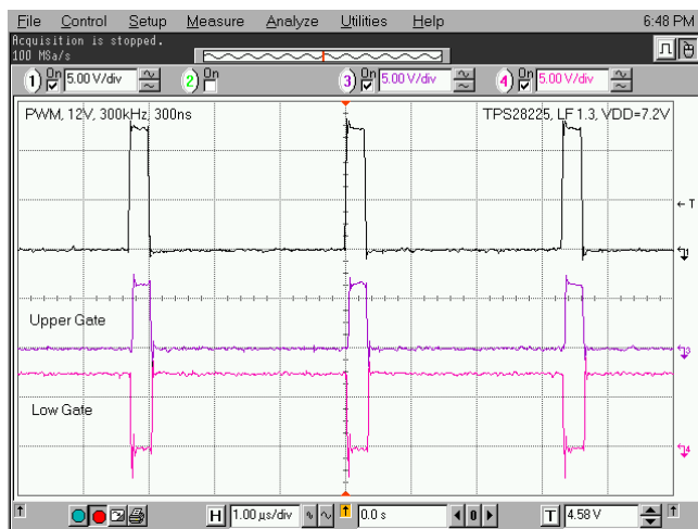
Figure 22. 12-V PWM Pulse at V_{DD} = 7.2 V
